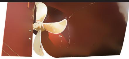
Bauer und Kaufman represents decades of experience in design and production of steering rudder blades for ships. All Rudders are made of carbon steel and are fully certified by DNVGL, LRS, ABS, BV, RINA. Full Databook with all material certificates included in every delivery.
